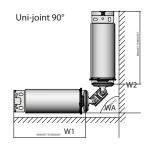
Uni-joint 45° and 90° brackets Maximum Roll Diametres: 40mm projection bracket: 75mm 55mm projection bracket: 105mm
