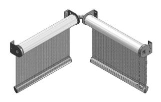
Uni-joint 45° and 90° bracketing systems allow blinds to remain linked in both manually and motorised Ambience multi-linked blinds. Uni-joint 45° brackets are suitable for the multi-linking of Ambience roller blinds between angles ranging from 0° to 45° out of parallel. Uni-joint 90° brackets are suitable for the multi-linking of Ambience roller blinds between angles ranging from 45° to 90° out of parallel. When ordering a uni-joint system:
